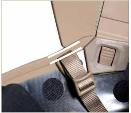
10-A. Ensure that the front strap end is parallel to the inside edge of the helmet. Tighten screw and anchor A. Proper torque value of screw/anchor A is 20 in-lb. Non-permanent thread locker may be applied to screw/anchor as necessary.
