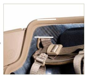
11. Double check the position of all the components: Rail, Chop/Ear, accessory mount, and helmet strap ends. Tighten screw and anchor C. Proper torque value of screw/anchor C is 6 in-lb. Non-permanent thread locker may be applied to screw/anchor as necessary. Replace impact pads if they were removed in Step 2.
