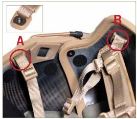
5. Place left Rail on exterior side of helmet. Ensure helmet straps are not twisted. Insert anchors A and B into strap ends. Secure Rail and straps to helmet. Loosely tighten screws A and B so that the Rail and strap ends are still movable and can be easily repositioned.
